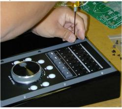
3. Carefully separate the top panel from the bottom panel of both units. Set aside top panels for reassembly.
