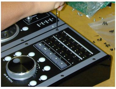
11. Replace and secure all screws in the bottom panel with a #1 Philips screwdriver.
