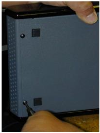
2. Remove six external screws (three along each side) from top of both units, using the supplied 5/64 inch hex driver and set aside for reassembly.
