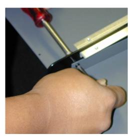
9. Replace the top metal for both units. During this time, it may be possible pass the data and/or power cables between the units by passing the cables through the two circular holes in the Eclipse Series Joiner. Consult the documentation of the specific Eclipse units or contact the JLCooper Service Department.
